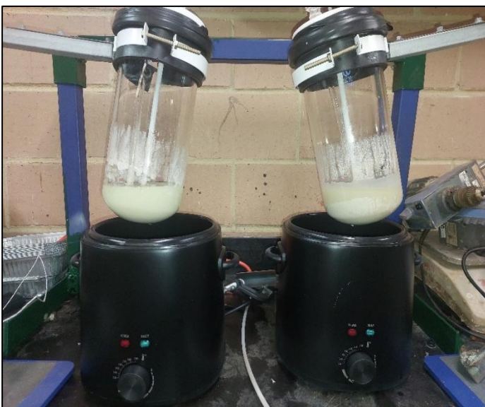
Image 7 Hydrolysis and precipitation of titanium in stirred glass reactor & Image 8 Precipitated \text{TiO}_2 .
