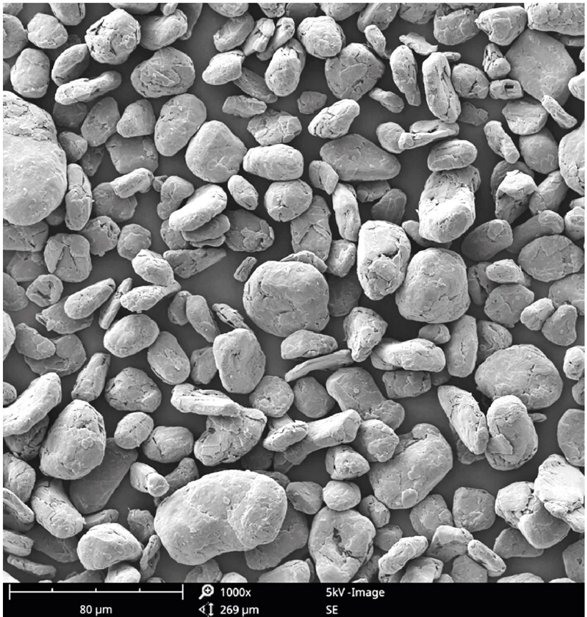
Figure 18: SEM image of reference material Ref 26; magnification 1,000x
