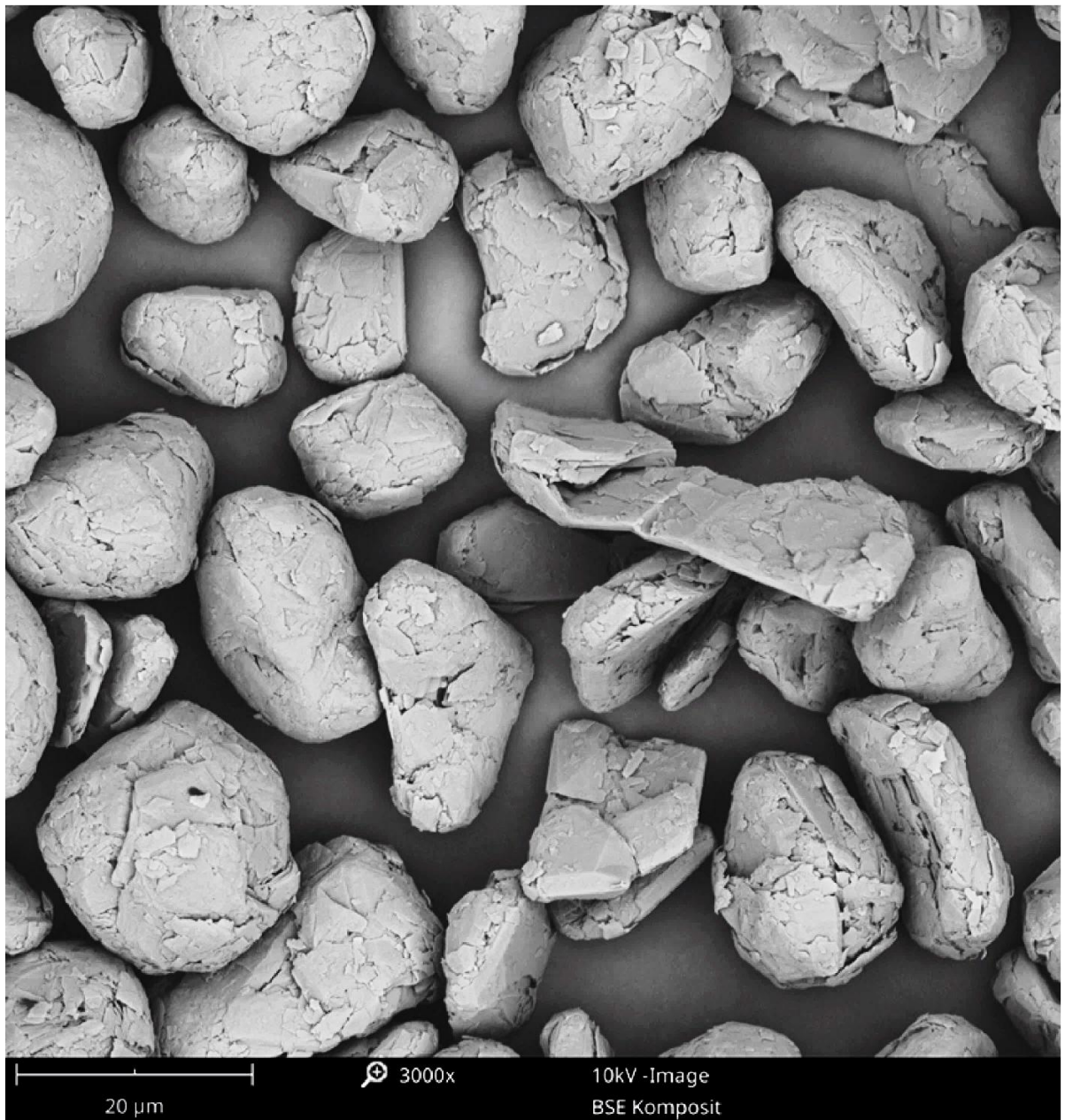
Figure 17: SEM image of reference material Ref 17; magnification 3,000x
