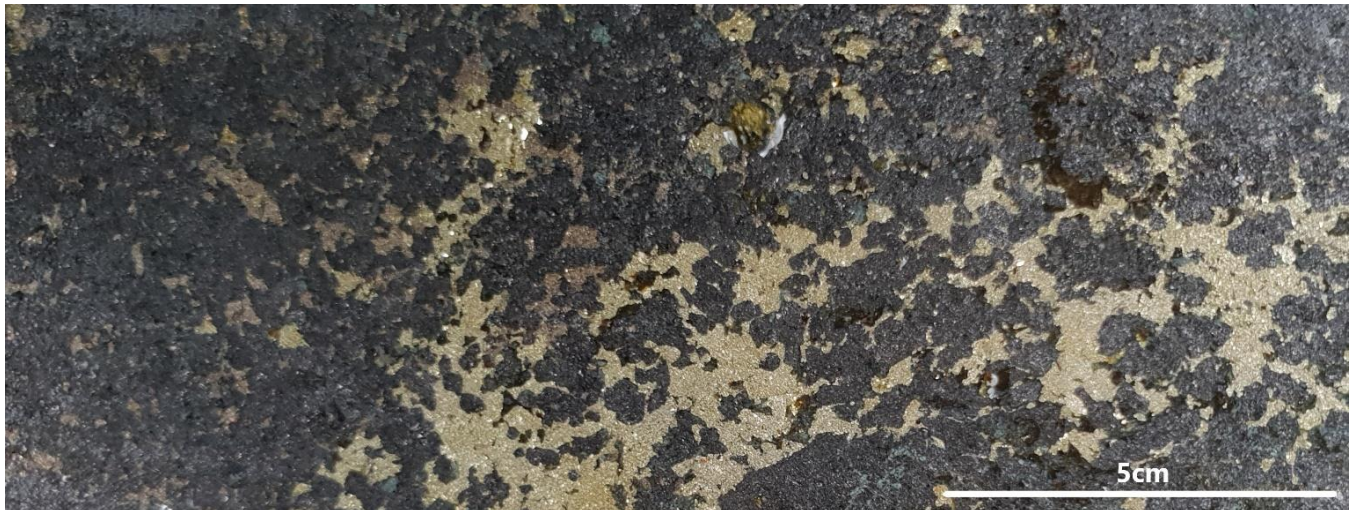
Image 1: MND003, 66.3m, magnetite- Ilmenite cumulate with interstitial sulphides (pyrite, pyrrhotite & chalcopyrite)
