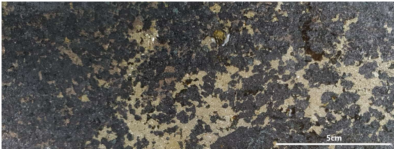
Image 2: MND003, 66.3m, magnetite-ilmenite cumulate with interstitial sulphides (pyrrhotite, pyrite, chalcopyrite)
