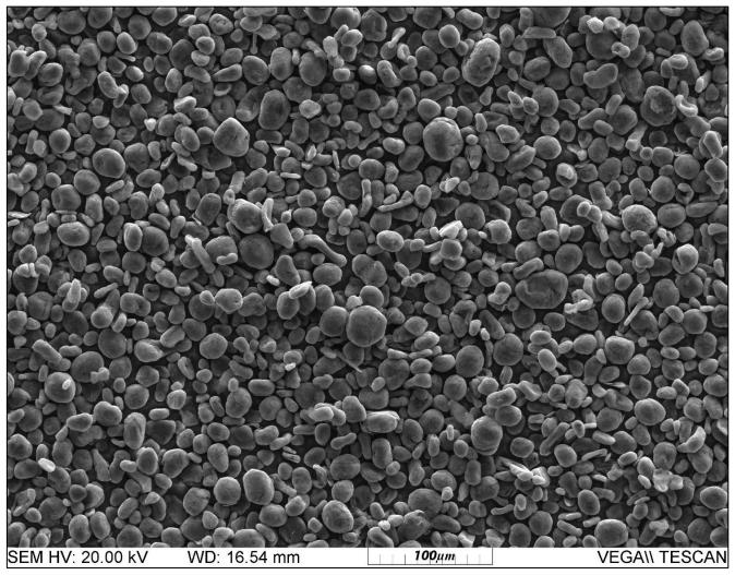
Image 1: Scanning Electron Microscope (SEM) image of Lac Rainy spherical graphite (average  $20\mu m$ )
