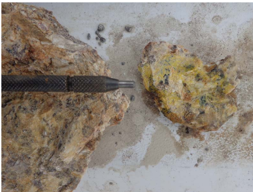
Figure 2. Alaskite with smoky quartz (black) and carnotite (light yellow). Smoky quartz is developed through damage to the quartz crystal structure through radioactive breakdown, most likely from primary uranium minerals rather than the secondary carnotite shown here.
