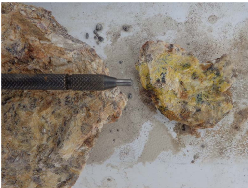
Figure 2. Alaskite with smoky quartz (black) and carnotite (light yellow). Smoky quartz is developed through damage to the quartz crystal structure through radioactive breakdown, most likely from primary uranium minerals rather than the secondary carnotite shown here.
