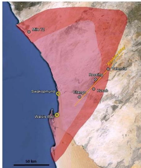
Figure 2 – Areas exhibiting prime geological conditions for the genesis of alaskites. Mile 72 had the same conditions as those experienced at Husab, Rössing and Valencia. (Red = peak conditions ideal for genesis of alaskite. Pink = peak conditions exceeded required conditions but area still hosts potential for alaskites.)
